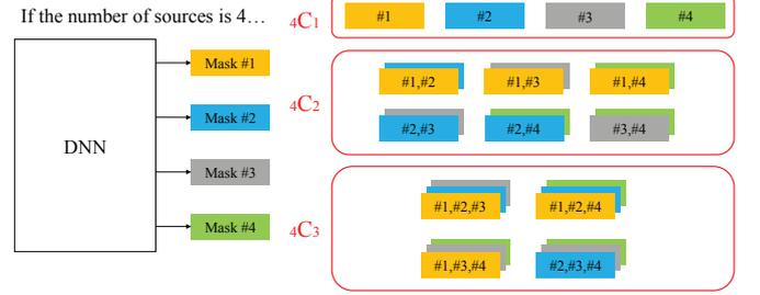
Fig. 2: Combination Loss (CL). To simplify, this figure is an example that the mixture input is consisted of 4 sources.
