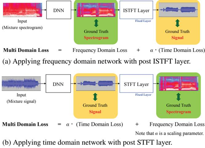
Fig. 1: Multi domain loss (MDL)
